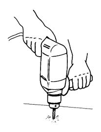
NOTE: The correct and SAFE way to drill.
