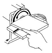
Note: To be safe, sand on the down stroke/left side only!
